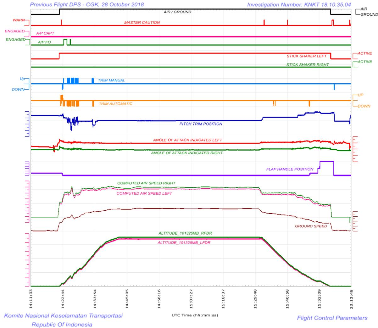
Figure 7: The significant parameters of the previous flight
